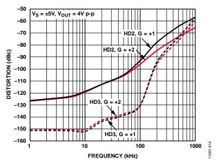
Figure 12. Distortion vs. Frequency for Various Gains
