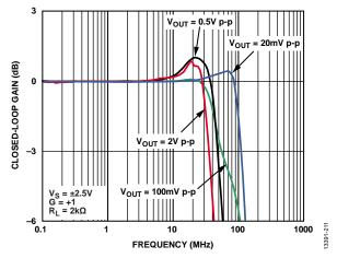
Figure 10. Frequency Response for Various Output Voltages
