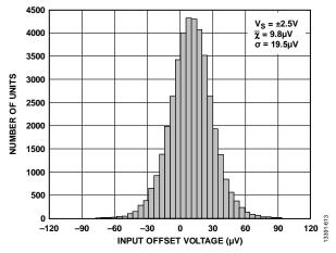
Figure 23. Input Offset Voltage Distribution
