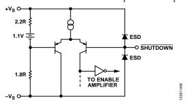
Figure 54. Shutdown/Sleep Equivalent Circuit
