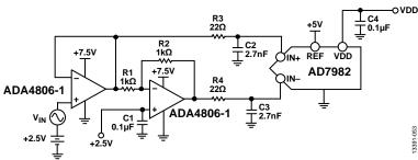
Figure 65. Driving the AD7982 with the ADA4806-1
