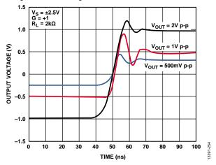
Figure 57. Step Response with Selected Output Steps
