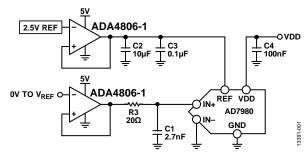
Figure 1. Driving the AD7980 with the ADA4806-1
