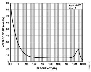
Figure 17. Voltage Noise vs. Frequency
