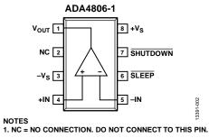
Figure 4. Pin Configuration
