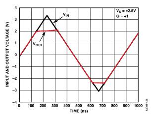
Figure 30. Input Overdrive Recovery Time
