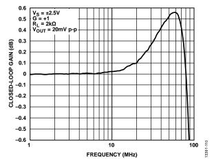
Figure 14. Small Signal 0.1 dB Bandwidth
