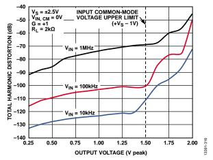
Figure 13. Total Harmonic Distortion vs. Output Voltage For Various Frequencies
