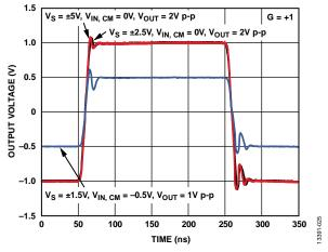
Figure 32. Large Signal Transient Response for Various Supplies
