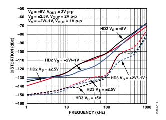
Figure 15. Distortion vs. Frequency for Various Supplies, G = +1
