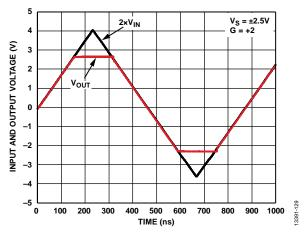
Figure 33. Output Overdrive Recovery Time
