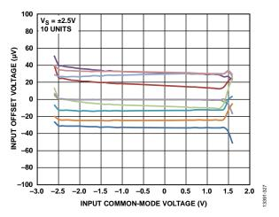
Figure 24. Input Offset Voltage vs. Input Common-Mode Voltage
