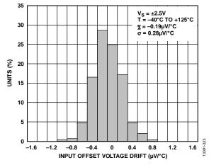
Figure 26. Input Offset Voltage Drift Distribution
