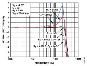
Figure 59. Peaking in Frequency Response at Selected R<sub>F</sub> Values
