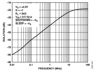
Figure 21. Forward Isolation vs. Frequency
