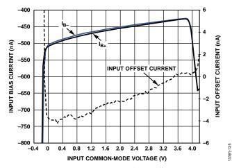
Figure 28. Input Bias Current and Input Offset Current vs.
