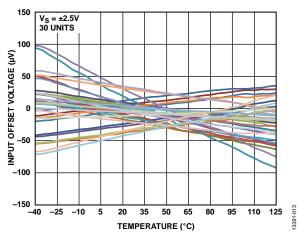
Figure 27. Input Offset Voltage vs. Temperature
