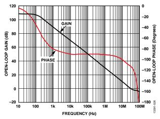
Figure 46. Open-Loop Gain and Phase Margin
