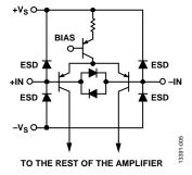
Figure 53. Input Stage and Protection Diodes
