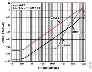
Figure 19. CMRR, PSRR vs. Frequency
