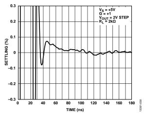
Figure 22. Settling Time to 0.1%
