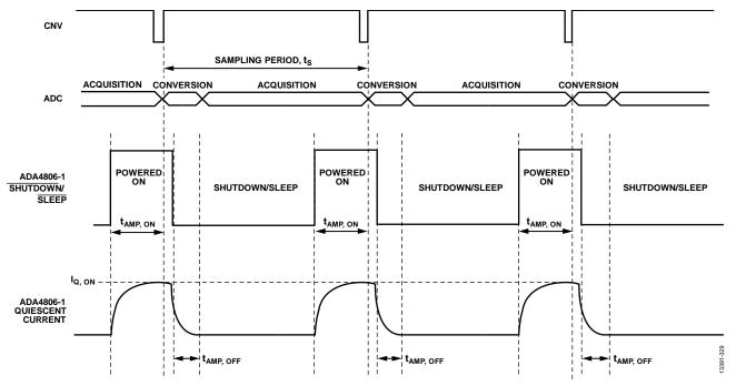
Figure 63. Timing Waveforms
