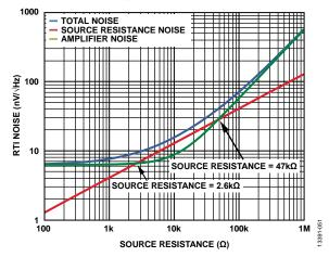
Figure 56. RTI Noise vs. Source Resistance
