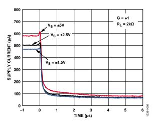
Figure 40. Turn-Off Response Time to Sleep for Various Supplies
