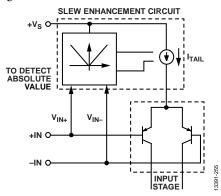
Figure 52. Slew Enhancement Circuit
