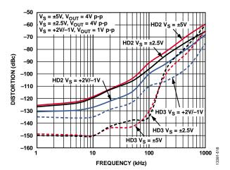
Figure 16. Distortion vs. Frequency, G = +2
