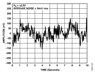
Figure 18. 0.1 Hz to 10 Hz Voltage Noise
